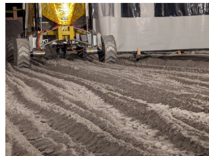
Figure 1: PRIMROSE after 30km driving on-lunar simulant
