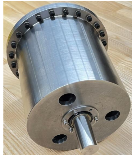
Figure 2: Assembled prototype cycloidal magnetic gear.
