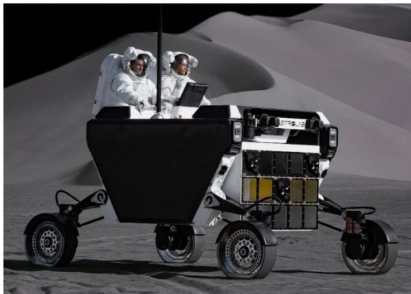
Figure 2: FLEX's modular payload interface and novel mobility system enable it to perform a multitude of functions, including crew transport, outpost logistics, robotic science, and infrastructure deployment
