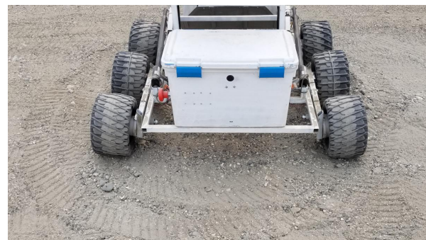
Figure 3: 6-wheel rover in radial slant grouser configuration, after four full rotations on gravel.
