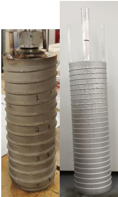
Figure 1. Thermal corer prototypes for ice extraction. Left: 17.3 cm long stainless steel based thermal corer; Right: 34.5 cm long aluminum alloy based thermal corer
