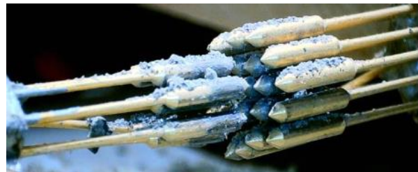
Figure 4. Amphenol's lunar brush contact prototype after 2,500 durability cycles (patent pending).
