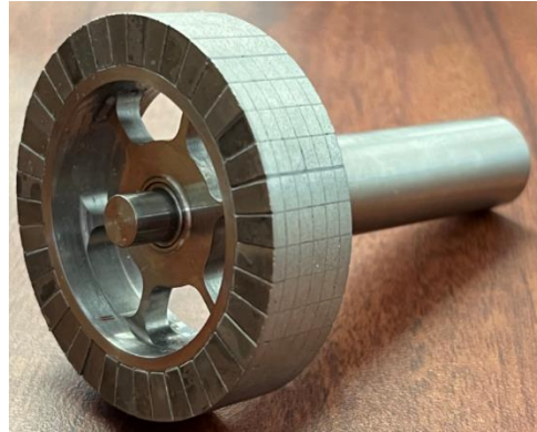
Figure 1: Sun gear for the proof-of-concept actuator's magnetically-geared motor.
